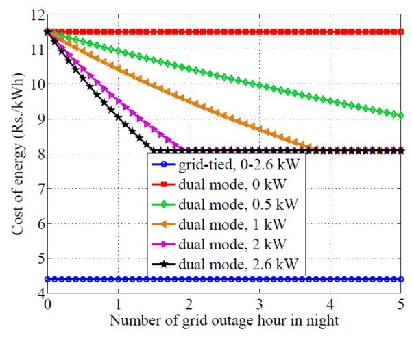
During night time grid outage, battery supplies critical loads till capacity saturation.
