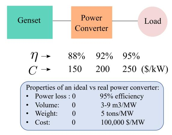
All the above trade-offs can be combined together to select the best power converter configuration for a given microgrid application
