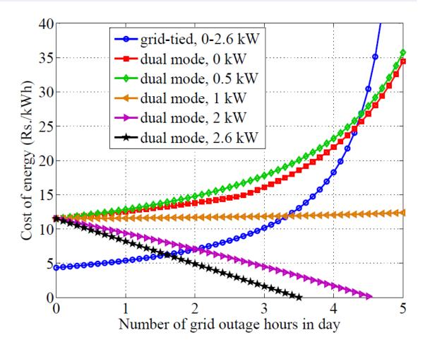
During day time grid outage, PV microgrids with storage are better with lower COE.
